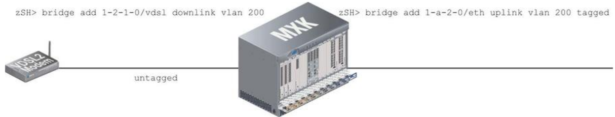
Figure 133: MXK to VDSL modem on untagged downlink
