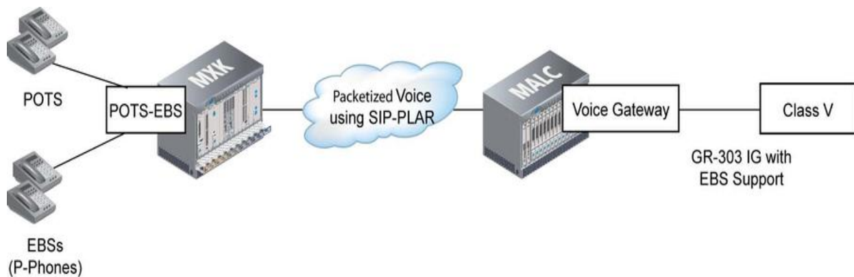
Figure 165: POTS-EBS card supports packet voice
