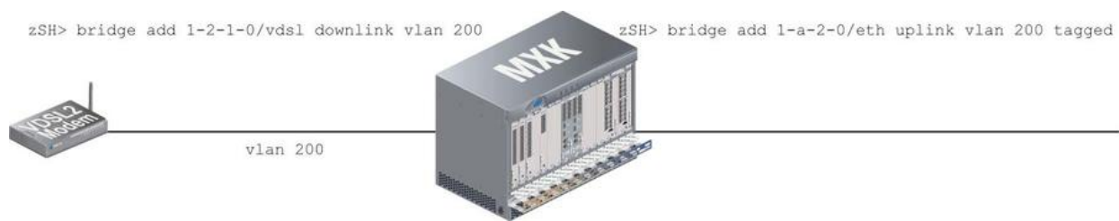
Figure 135: MXK to VDSL modem on tagged downlink
