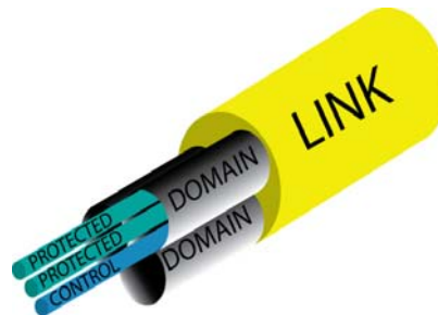
Figure 90: With multiple VLANs on a link one is a control VLAN which protects the other VLAN
